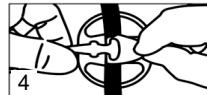
Pull the tip of the strap through the slit in the device Caution: Do not overtighten
